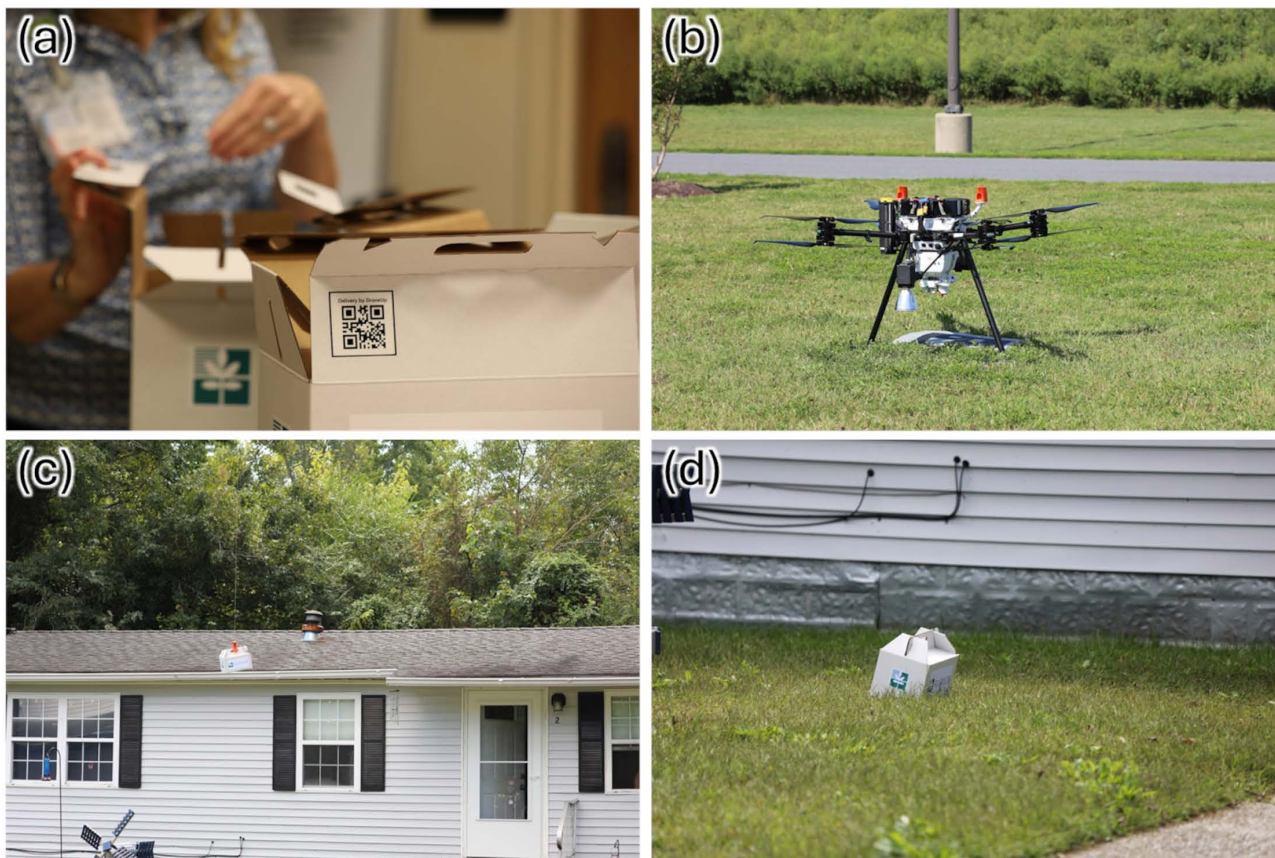
Fig 2. Stages of drone delivery of hypertension medications to patients on the Eastern Shore of Virginia: (a) Medications are prepared and packaged by a healthcare professional; (b) the drone is loaded with the package and a charged battery; (c) the medication is lowered to the patient's residence using a winch line; (d) the package is left on the lawn for the patient to retrieve. Photos Courtesy of Virginia Institute for Spaceflight & Autonomy as part of the Elevating Healthcare Access Project.
