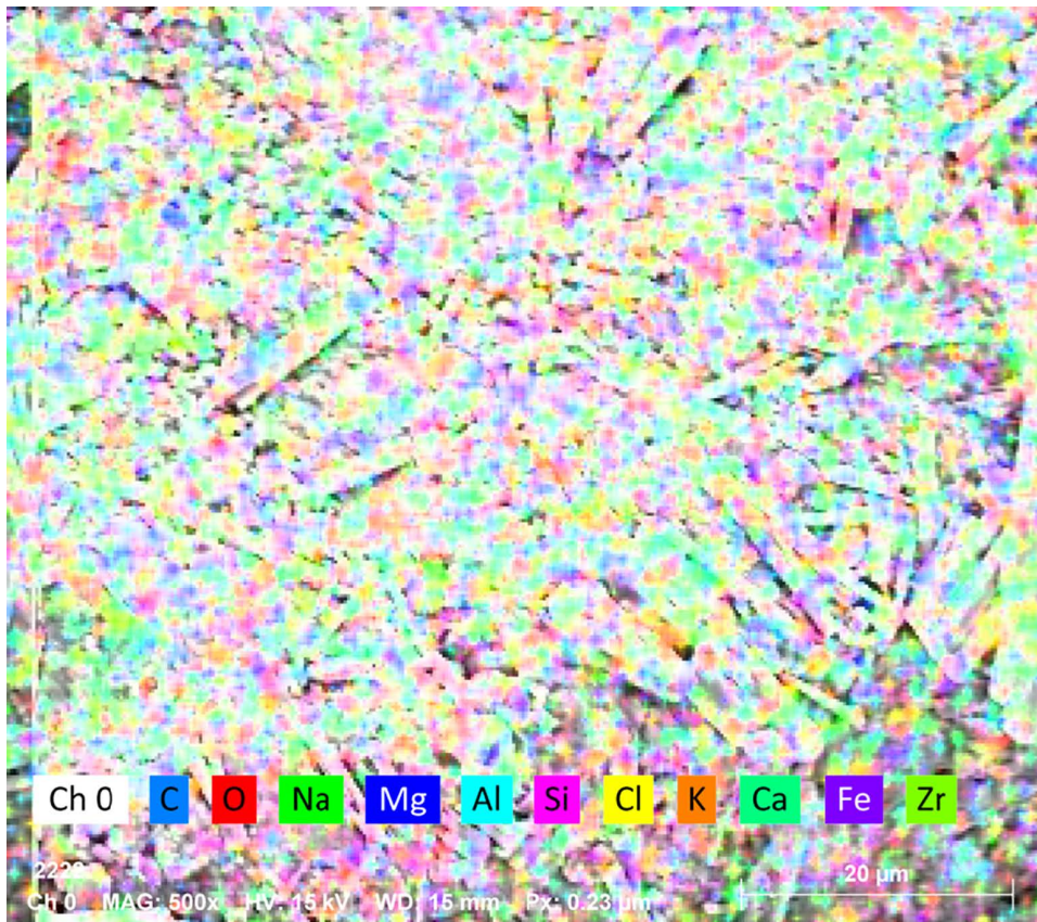
Fig 18. Elemental composition and quantitative results. Detected elements (ordered by energy): C, O, Na, Mg, Al, Si, Cl, K, Ca, Fe, Zr, Light elements (C, O): Potential sample constituents or surface contaminants, Na-Al-Si group: Typical of silicates or aluminum alloys, Fe-Zr: Possible alloy components or ceramic phases (e.g., \text{ZrO}_2 ), Quantitative data: Dual values represent weight % and atomic % (e.g., 1.5 wt%/ 3.9 at%), Local variations (1.7%/2.6%) indicate phase heterogeneity.
