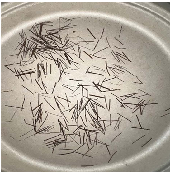
Fig 4. Physical morphology of raw palm fiber before mixing, showing typical yellowish-brown surface texture and fibrous bundle structure.
