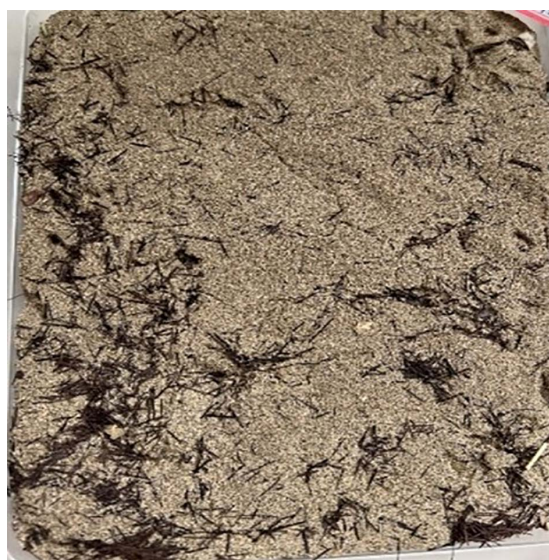
Fig 5. Surface appearance of MICP-treated sand sample after 7-day curing with 0.15% palm fiber content, demonstrating crust formation and structural integrity.
