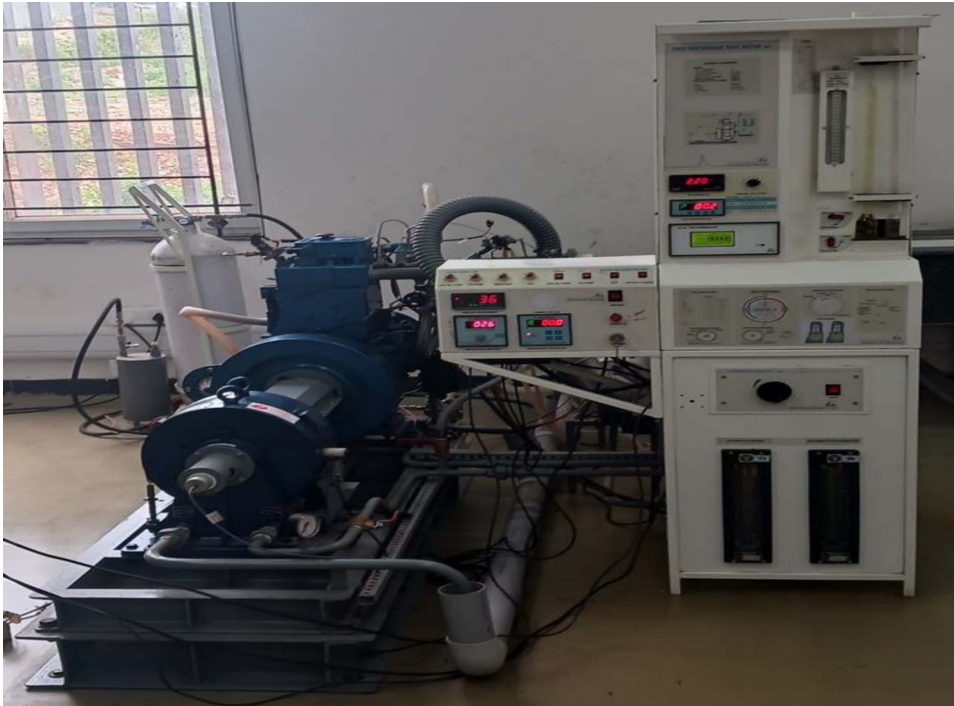
Fig 1. Computerized variable compression ratio diesel engine.
