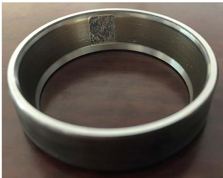
Fig 11. Damage to Ring of Bearing the outer ring of the bearing.
