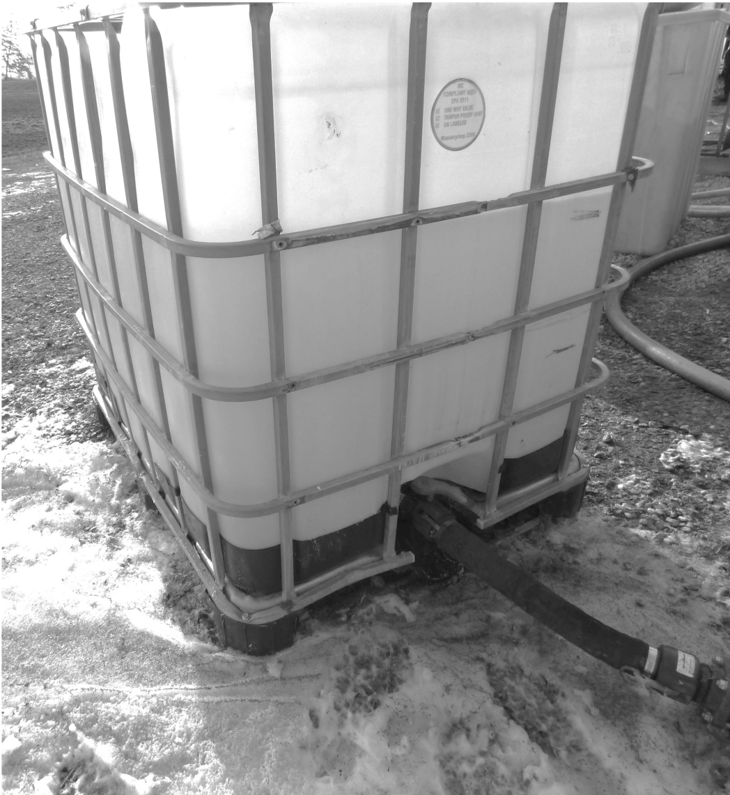
Fig 1. Intermediate bulk container (1136 L) with bottom drain used to mix foam-water solutions at prescribed concentrations. Fluid was pumped directly from container during foam production.
