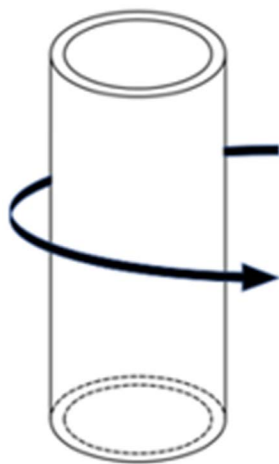
Fig 11. Hoop direction in steel tube.
