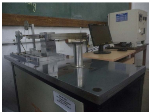
Fig 4. Image of Pin on disc setup.
