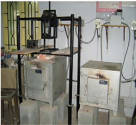
Fig 3. Stir casting setup with furnace.
