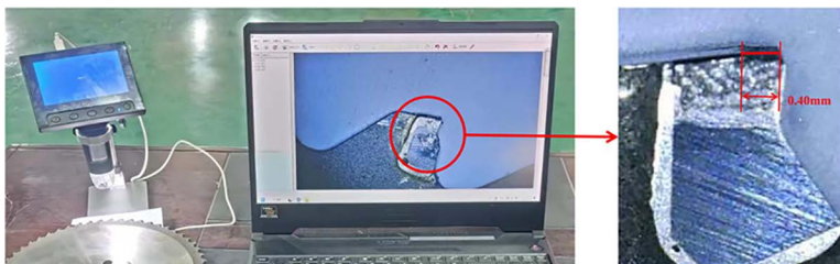
Fig 16. Measurement of saw blade wear value.
