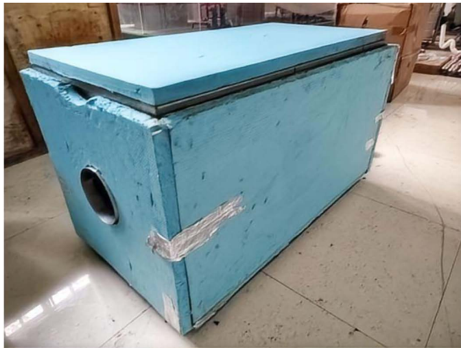
(c) Phase change energy storage heat exchanger overall package diagram
