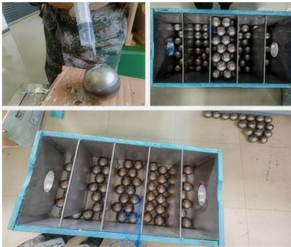
(b) Encapsulation of phase change energy storage heat transfer spheres and insulation of phase change energy storage heat transfer devices
