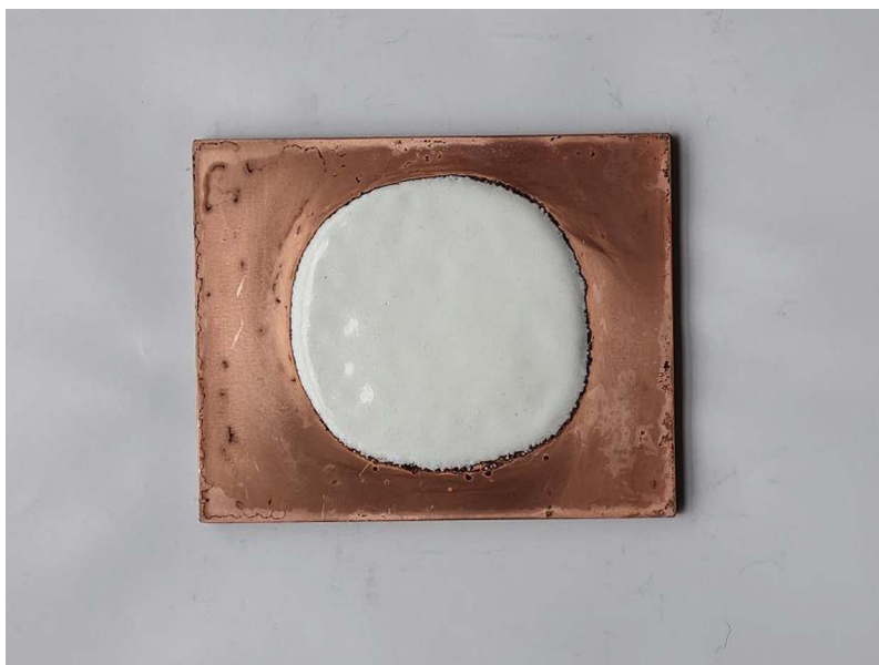
Fig 7. Enamel firing effect of larger porcelain-white enamel specimens.
