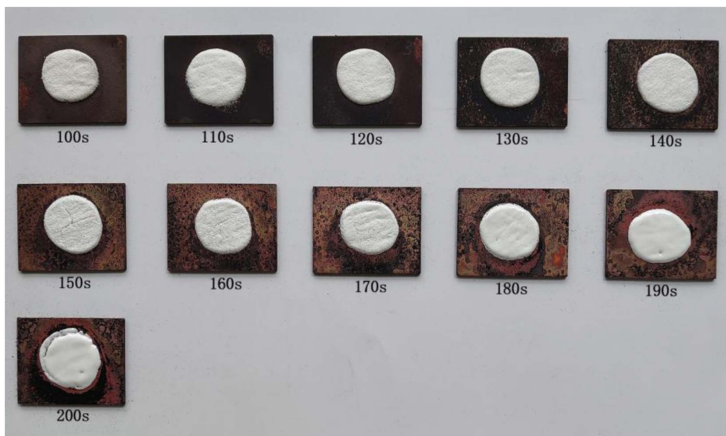
Fig 3. Enamel decorations of specimens 1 fired for different durations.
