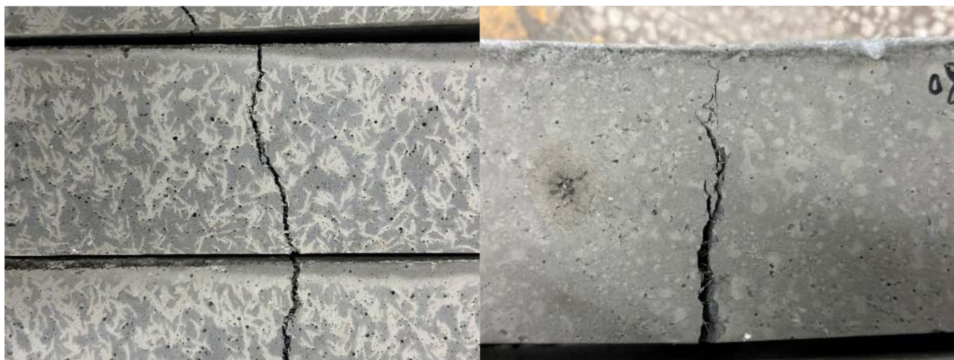
Fig 6. Concrete flexural failure pattern.
