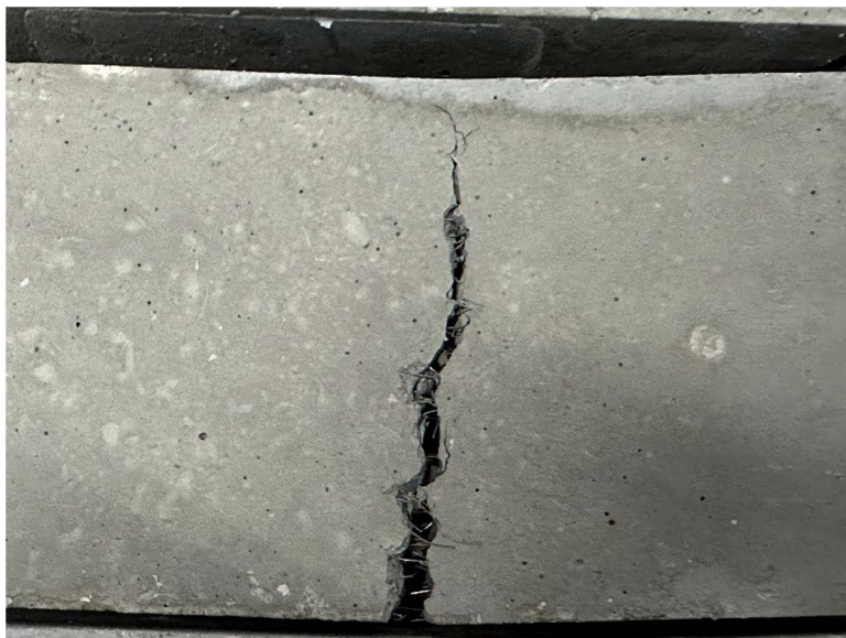
Fig 8. Elastic Modulus test loading of self-compacting steel fiber concrete.
