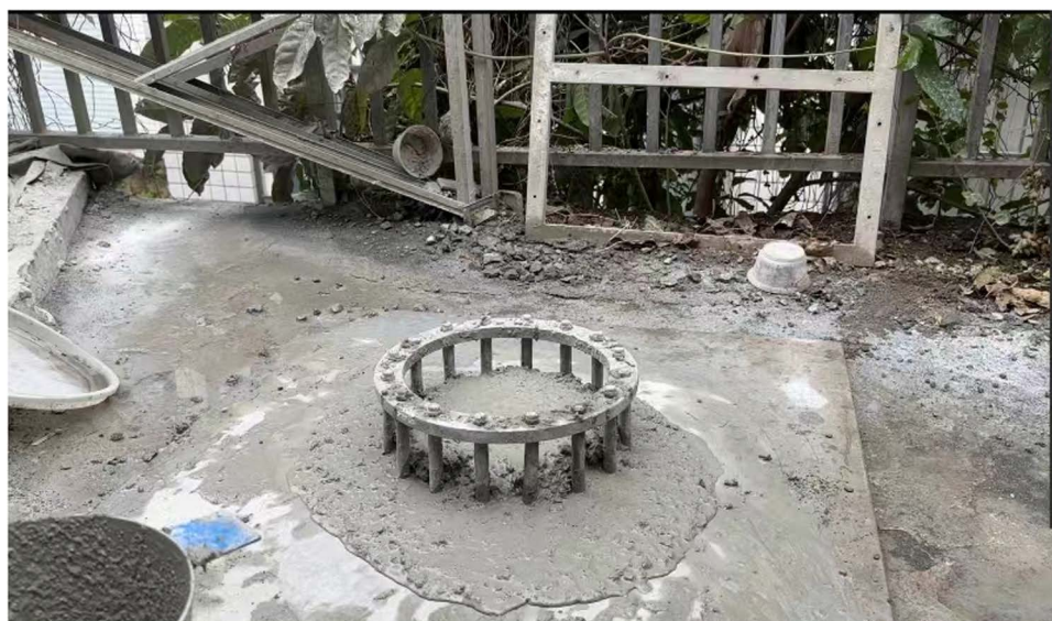
Fig 2. Slump expansion of steel fiber self-compacting concrete.
