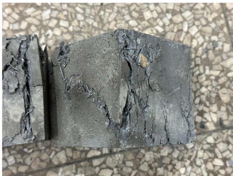
Fig 4. Compression failure pattern of concrete cube specimens.
