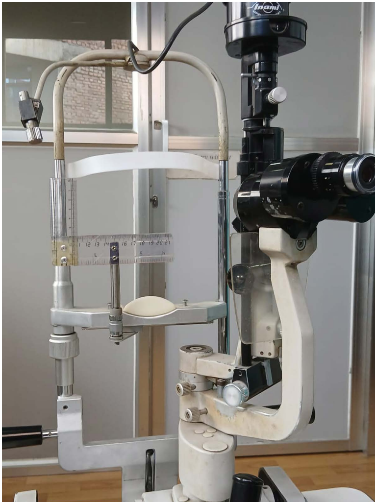
Fig 1. Customised slit lamp to measure implant and prosthesis motility.
