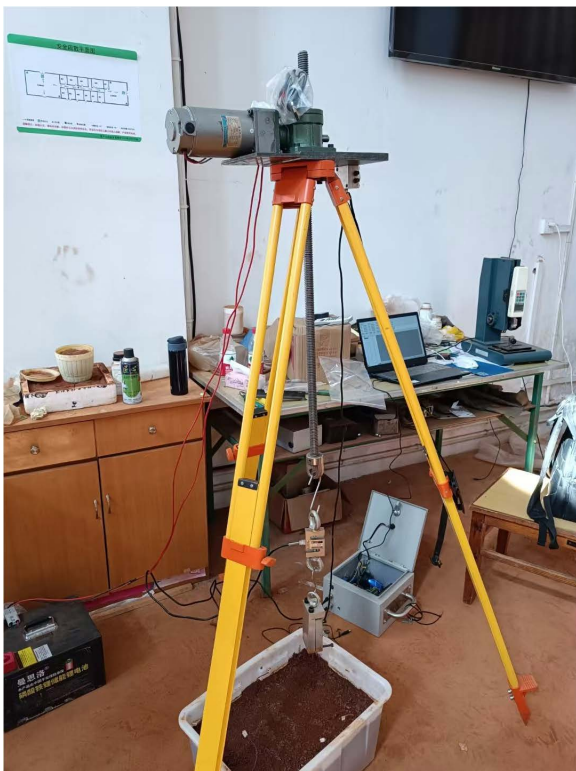
Fig 3. Schematic of the pull-out test apparatus.
