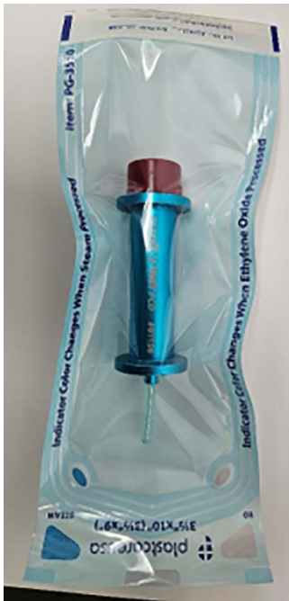
Fig 2. ePCD within sterilization pouch and placed alongside the load in the sterilization chamber.
