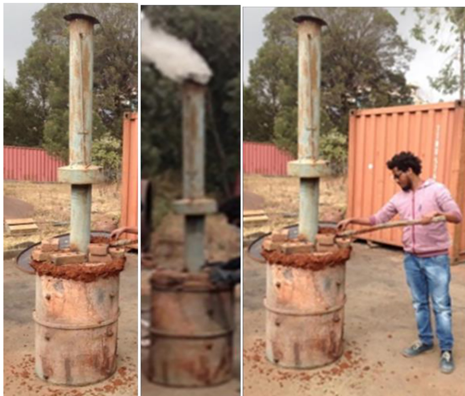
Fig 1. Drum Kiln for carbonization of Khat.
