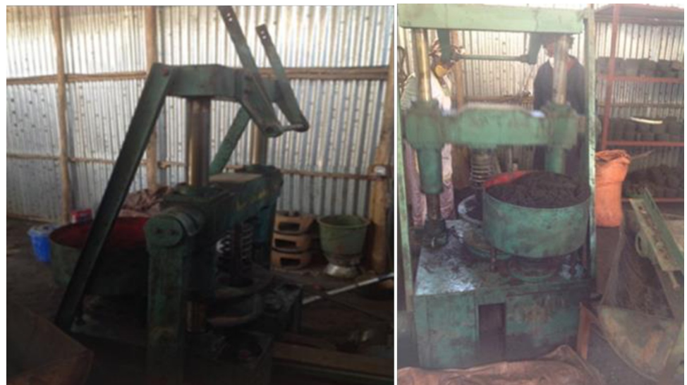
Fig 2. Beehives briquetting machine.
