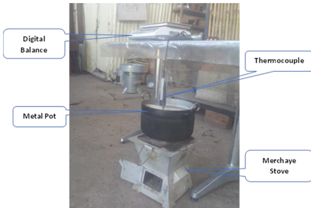
Fig 3. Water boiling test on produced Khat residue briquettes.
