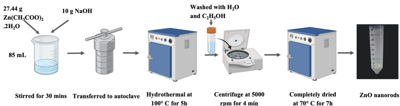
Fig 1. The schematic of ZnO nanomaterials preparation using the hydrothermal method.
