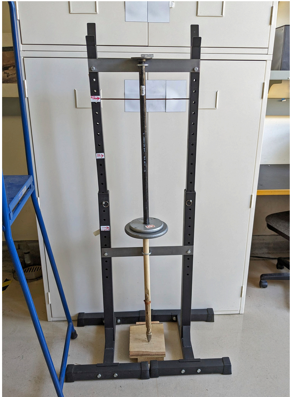
Fig 14. Replica 4 positioned between 8.1 kg drop weight and an oak plank in the freefall drop tower used in experiments phase I-III at Bear Bones Lab, UC Berkeley.
