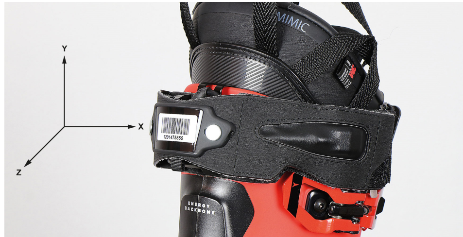
Fig 1. IMU attached to the ski boot via a strap.
