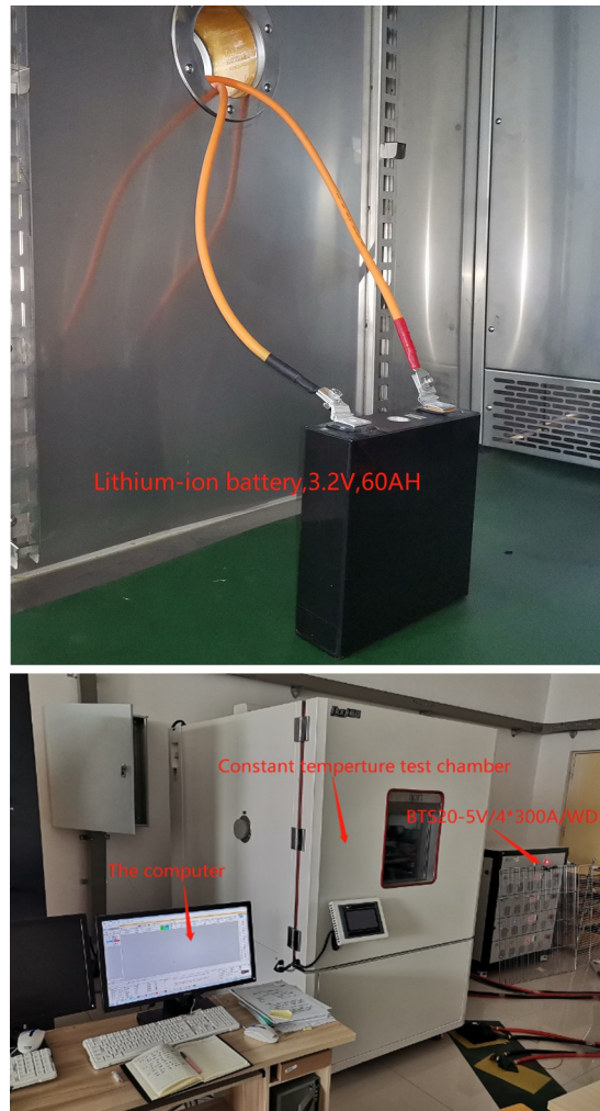
Fig 4. Battery testing system. (a) The lithium-ion battery. (b) The charge/discharge experiment (BTS20).
