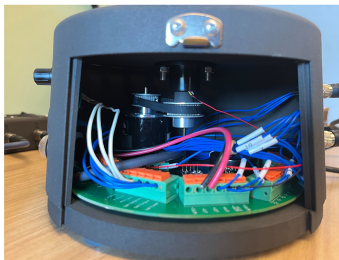
Fig 7. Interior components of the Perceptual Crossing Device controller.
