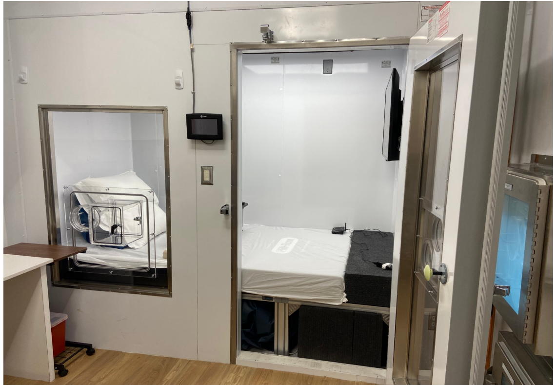
Fig 1. The small volume “flex” metabolic chamber at the Fralin Biomedical Research Institute at Virginia Tech Carilion in Roanoke, Virginia, set up for a resting measurement.
