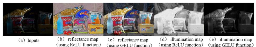
**Fig 5. Comparison of ReLU function and GELU function in decomposition network.**
