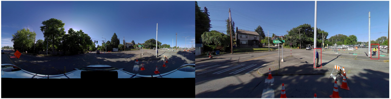
Fig 1. Sample images from the pedestrian detection data pipeline. The left image is an original 360° image from a data collection run. The image on the right is the right-hand side of the original image after orthorectification and pedestrian detection (both sides of the image are processed separately). There are two pedestrians that were detected by the algorithm (in red bounding boxes).
