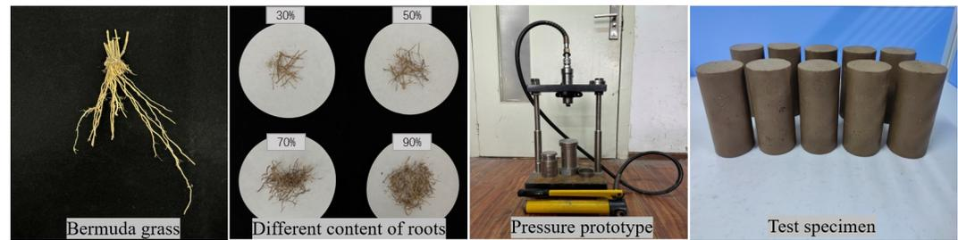
**Fig 3. The Sample preparation process.**
