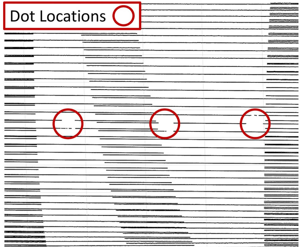
Fig 8. Laser scanner data with regions of missing data corresponding to dot locations highlighted.
