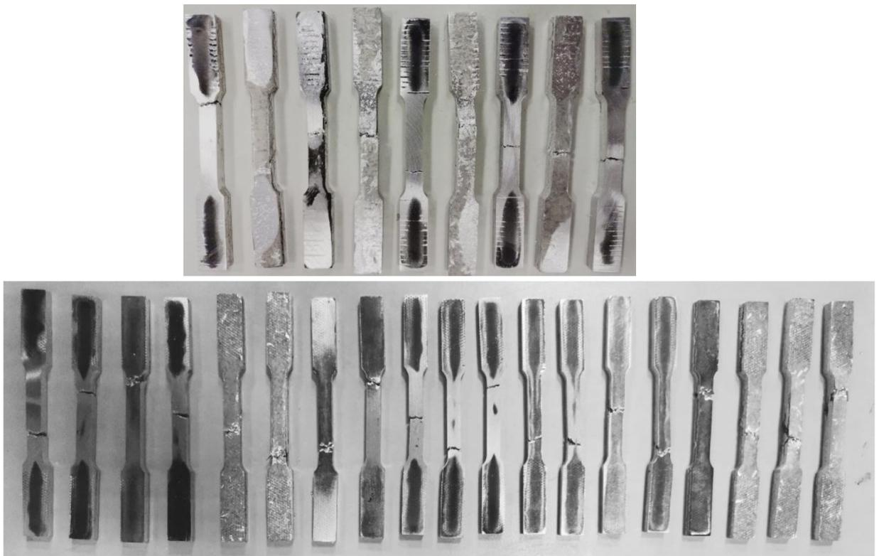
Fig 5. Recycled samples after tensile test.
