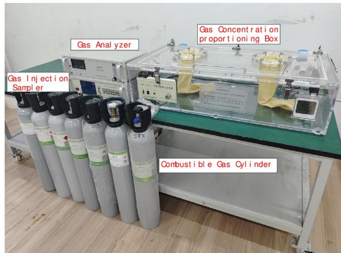
**Fig 7. Combustible gas concentration proportioning device diagram.**
