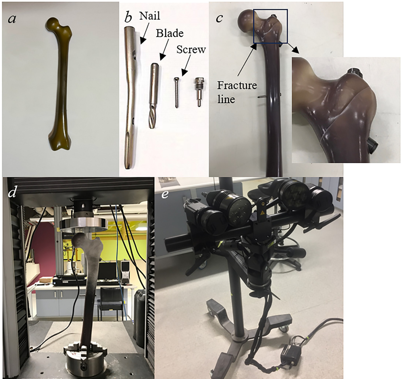
Fig 2. Mechanical testing of the (a) composite femur, (b) PFNA, (c) composite femur stabilized with PFNA, (d) INSTRON machine, (e) 3D optical ARMIS system.
