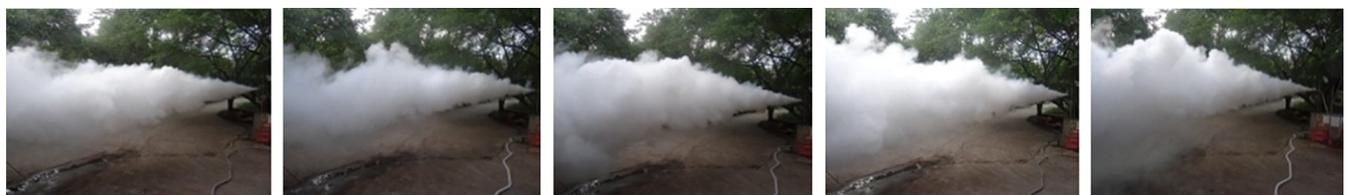
Fig 18. Comparison of jet conditions for different nozzles. (a) Adjustable, (b) 16 mm in diameter, (c) 21.5 mm in diameter, (d) 28 mm diameter, (e) No any nozzle.
