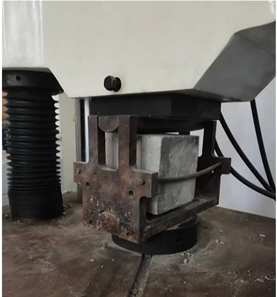
Fig 4. Split-pull loading device.
