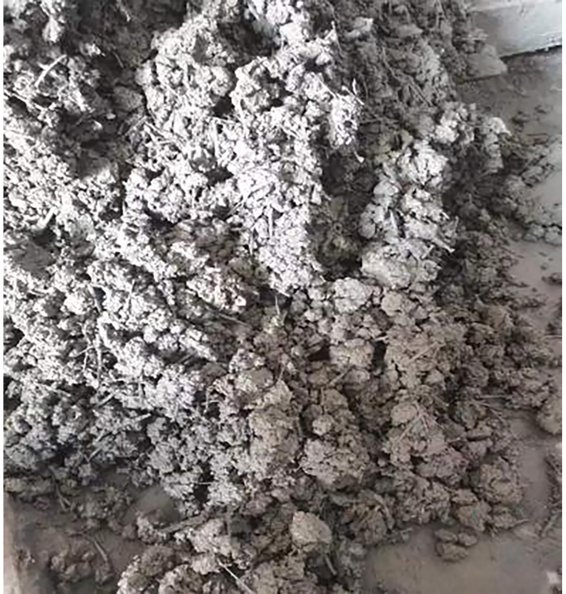
Fig 5. Steel fiber reinforced concrete mix.
