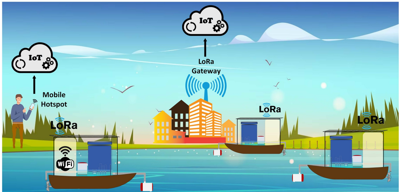
Fig 11. An extension of current work with more sensors and a few water quality systems distributed in water body, enabled with long range communications.
