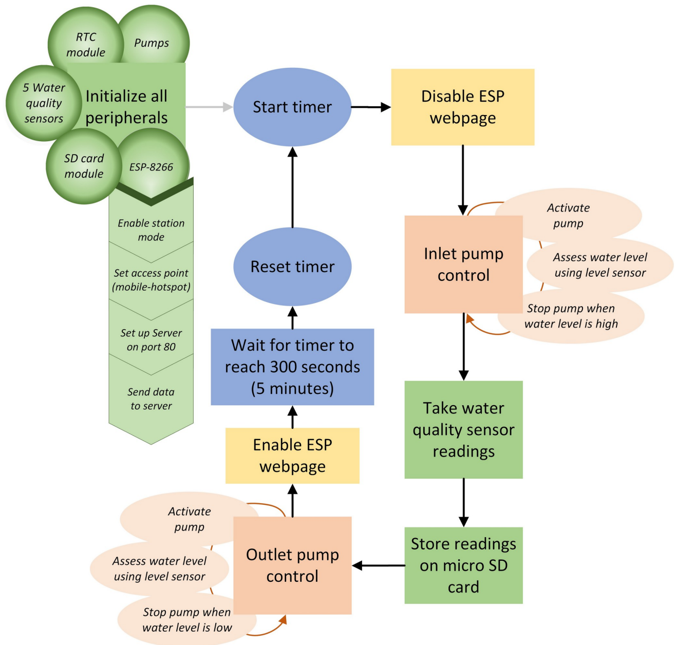
Fig 5. The flow chart illustrates the process of water sampling, sensor reading, and datalogging.
