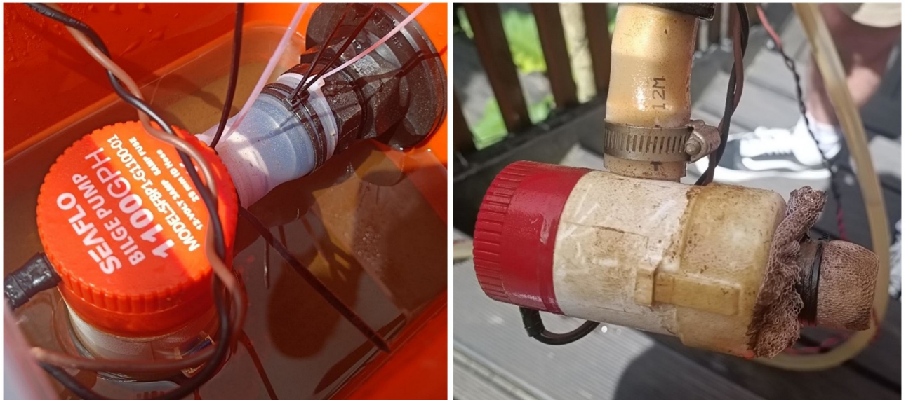
Fig 10. (left) sediment in water sampling tank, (right) small amount of dirt on inlet pump.
