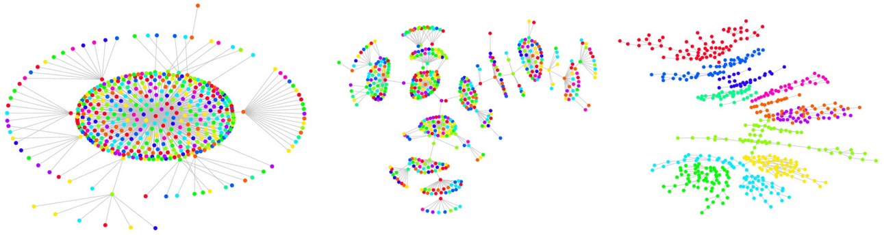
Fig 11. Minimum Spanning Trees (MSTs) obtained from the modified Vicsek generative model with varying \eta values: We generated MSTs using the modified Vicsek generative model with different values of \eta : (a) \eta = 0.010 , (b) \eta = 1.0 , and (c) \eta = 100.0 . The number of steps was set to 10000, and \delta was fixed at 0.10. For \eta = 100.0 , the vine structure is apparent and we used these vines to define the analogs of sectors in stocks. In particular, we performed a community finding on MST [33] corresponding to the vine structure, and identified 11 communities corresponding to the number of GICS sectors. These communities indeed constitute individual vines, as shown by colored nodes in the right-most figure. Next we tracked the associated stocks as \eta decreased based on the fixed \delta condition. Notably, as \eta decreases, the sectors collapse due to the fixed neighborhood of \delta , which encourages more particles (stocks) to interact with one another. This increased interaction arises as the particles experience less perturbation from \Xi , leading to homogeneous behavior and radial MSTs.
