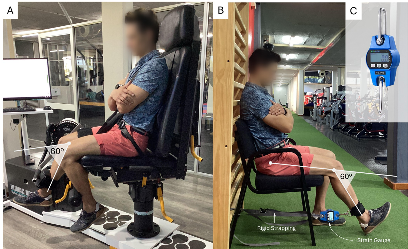
Fig 1. Experimental setup for the isokinetic dynamometer (panel A) and the strain gauge (panel B) for the right leg of a representative participant. The inset of panel C is a close-up of the commercially available strain gauge used in the study.
