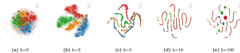
Fig 2. The t-SNE visualization of node features in DBLP dataset under different filter orders ( k = 0, 2, 5, 10, 100 ).
