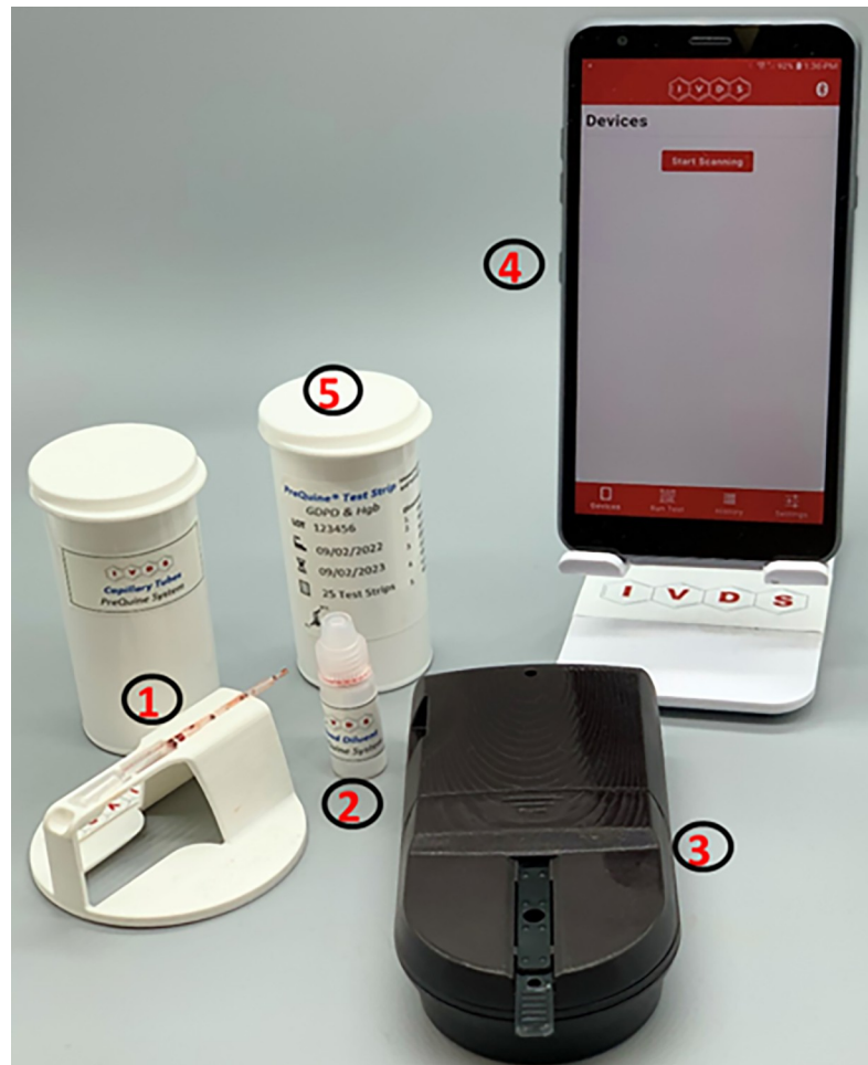
Fig 1. The PreQuine Platform consists of the following (1) Blood collection kits with single-use, fixed-volume pipettes, (2) Lysis buffer, (3) Handheld reflectance-based meter, (4) Cell phone application, and (5) Test strips for G6PD and Hgb detection.
