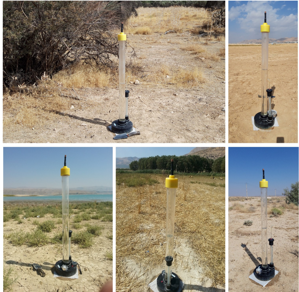
Fig 1. Measurement of K_{\psi} by tension-disk infiltrometer at different land uses.
