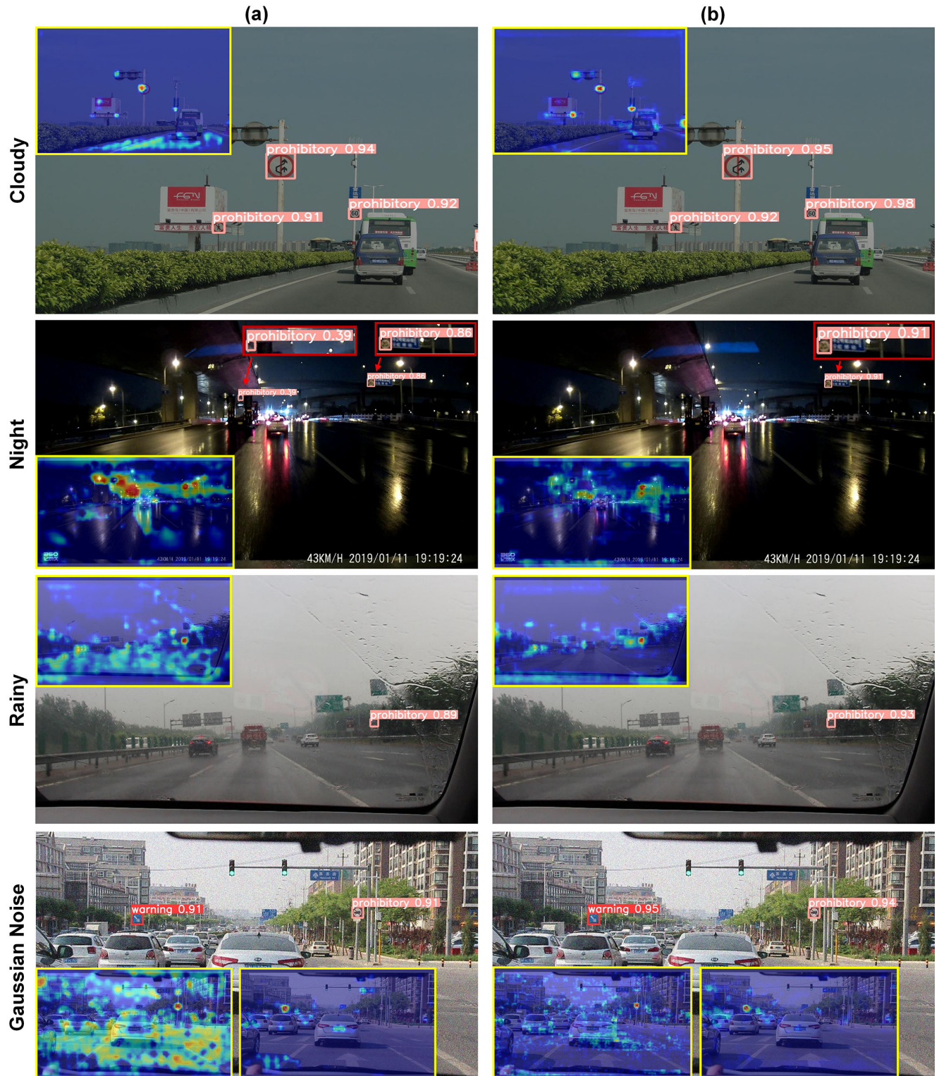
Fig 12. Sample test results using YOLOv5s and ETSR-YOLO in different scenarios. (a) is the test results of YOLOv5s. (b) is the test results of ETSR-YOLO.
