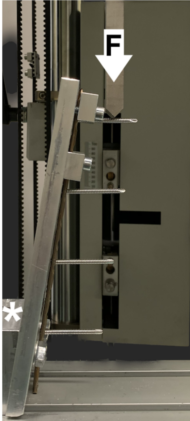
Fig 4. Set-up configuration. *displacement speed 1mm/min.
