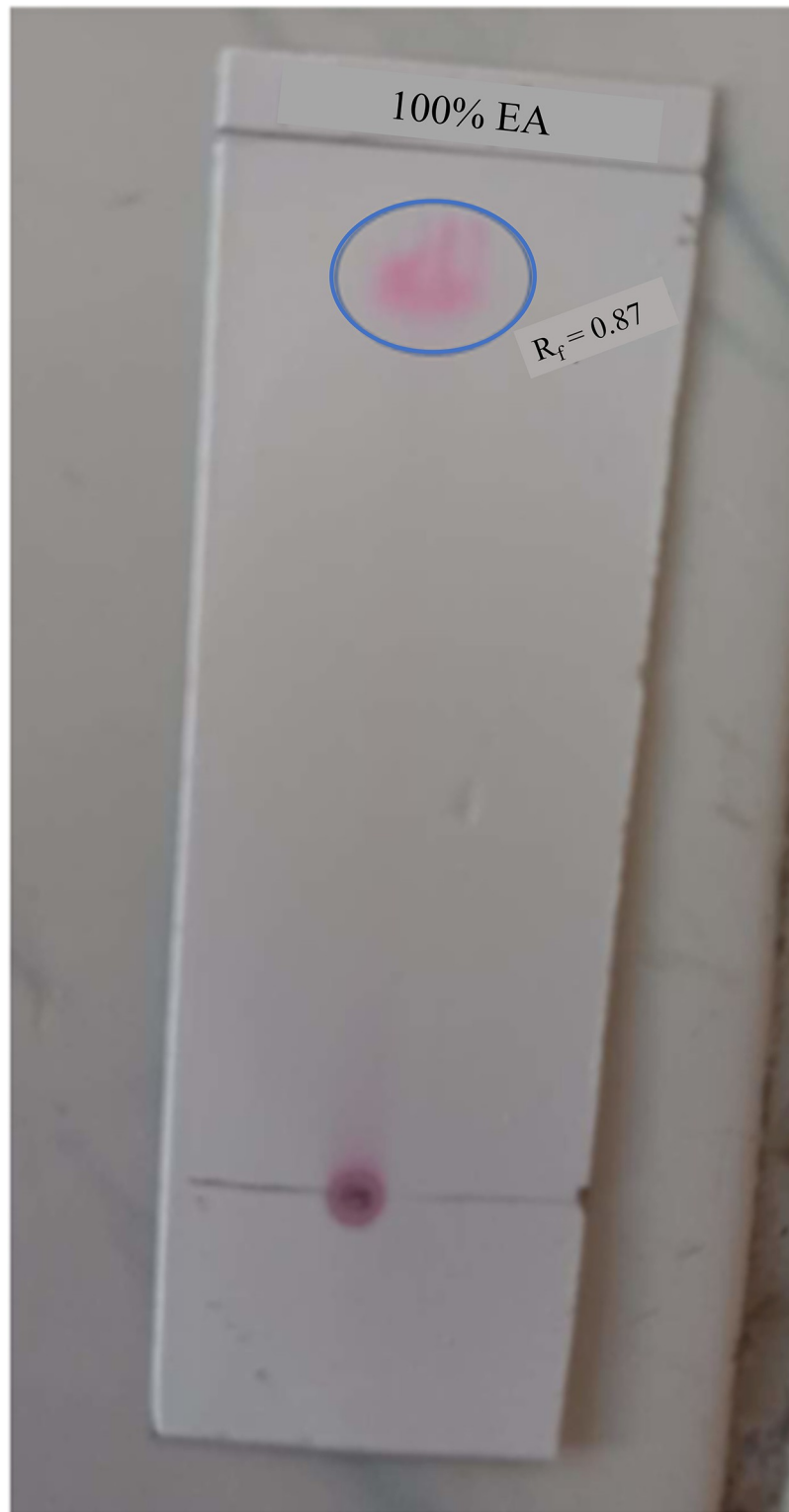
Fig 3. Chromatographic analysis of prodigiosin by Thin Layer Chromatography (TLC) showing R f value 0.87.
