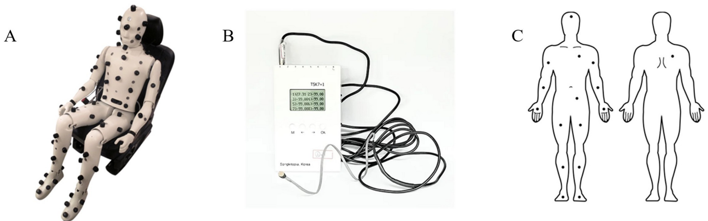
Fig 2. The measuring equipment. (A) The thermal manikin for the environment measurement. (B) The sensor and data logger for the skin temperature measurement. (C) The 16 body parts where the skin temperature sensors were attached.
