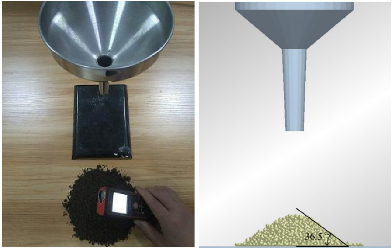
Fig 8. Parameter comparison experiment. (a) Real soil testing. (b) Simulated soil testing.
