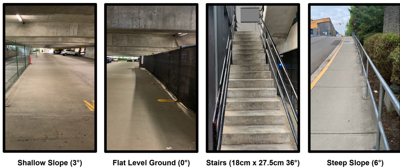
Fig 2. Terrain conditions used in the experiment. A total of seven conditions were collected including ascending and descending for the slope and stairs, and the flat ground condition.
