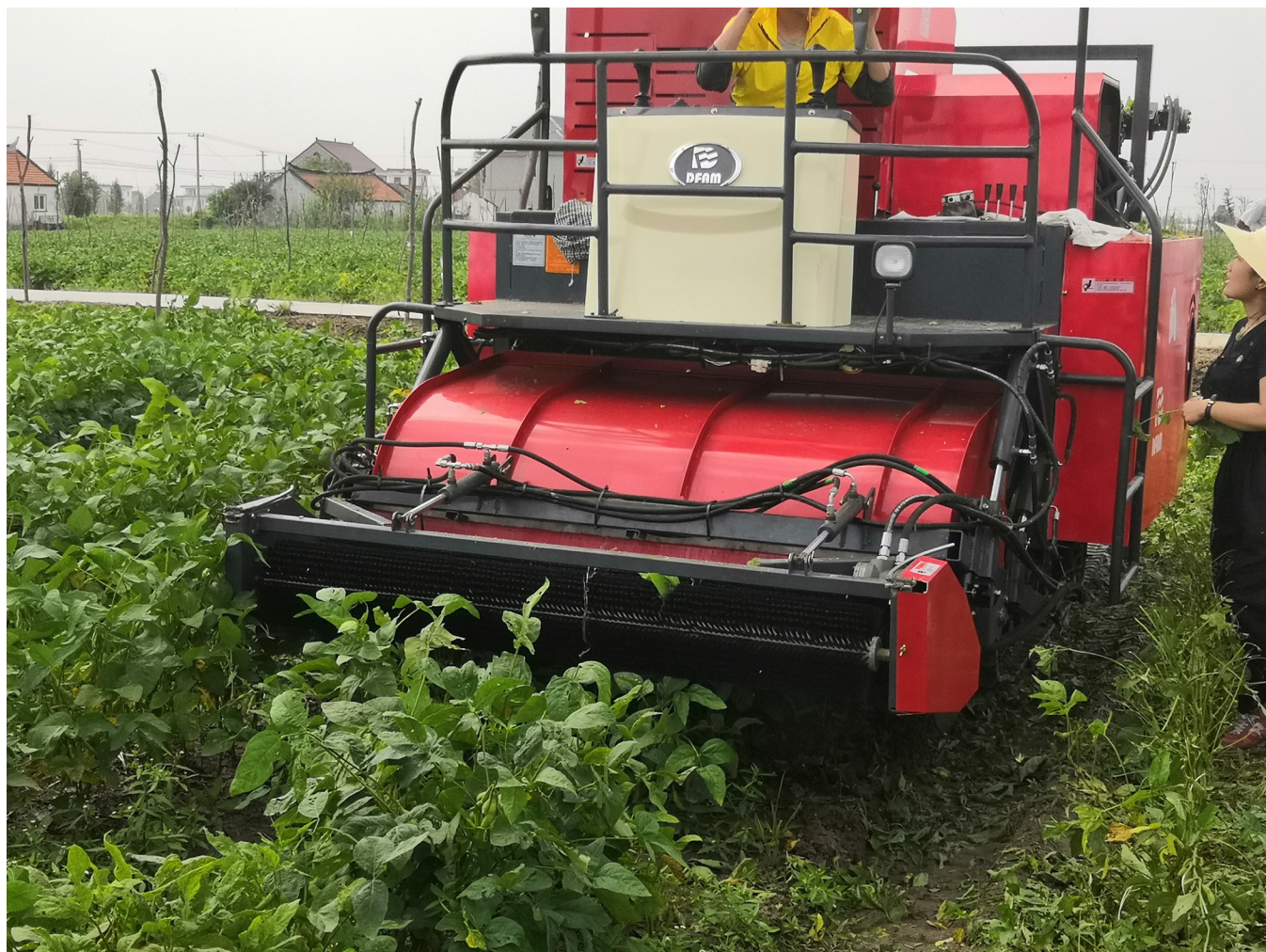
Fig 21. Field test of 4GQD-160 type self-propelled green soybean harvester.
