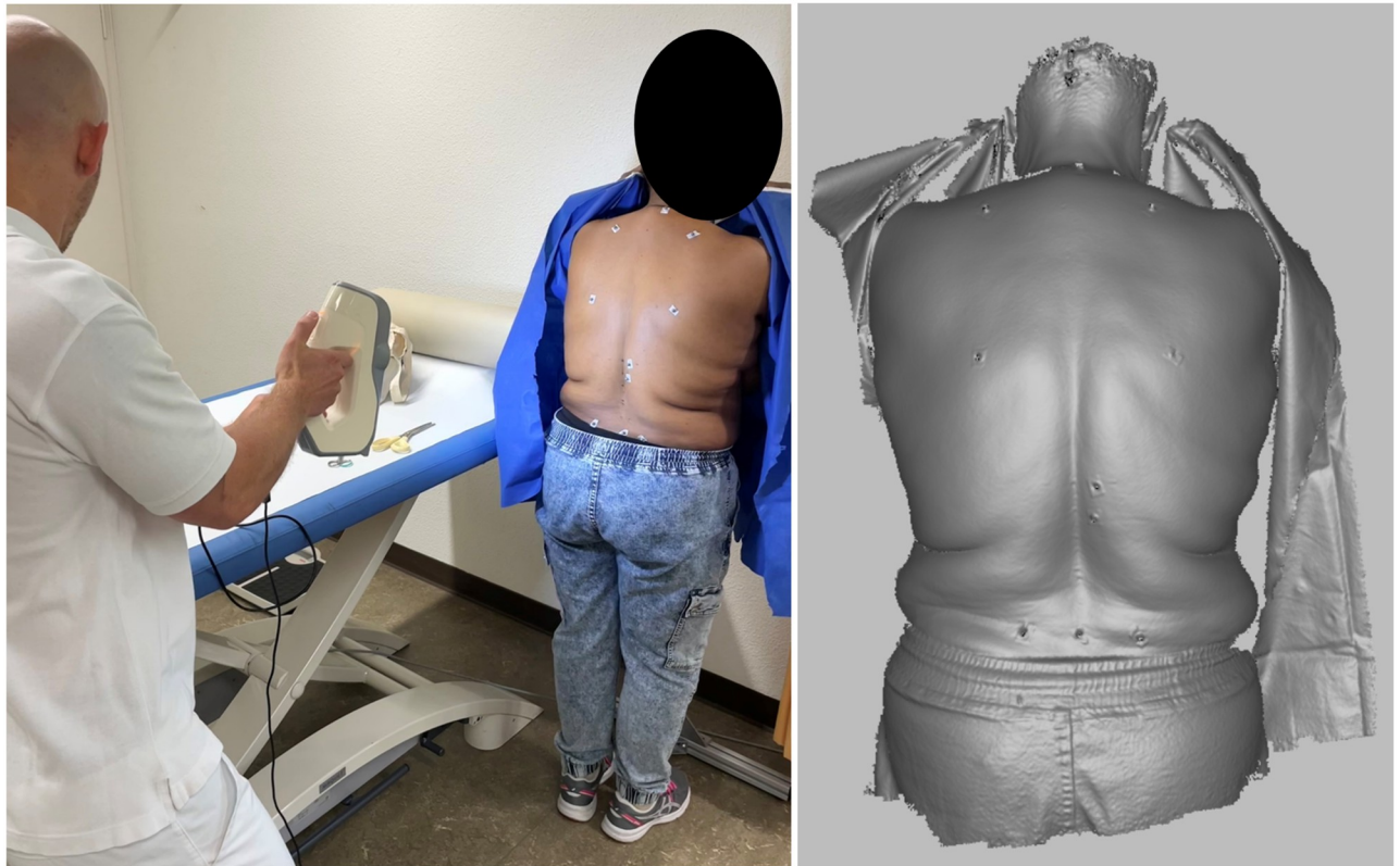
Fig 7. 3D optical digitalization with Artec EVA, https://www.artec3d.com , process (left), software output (right).
