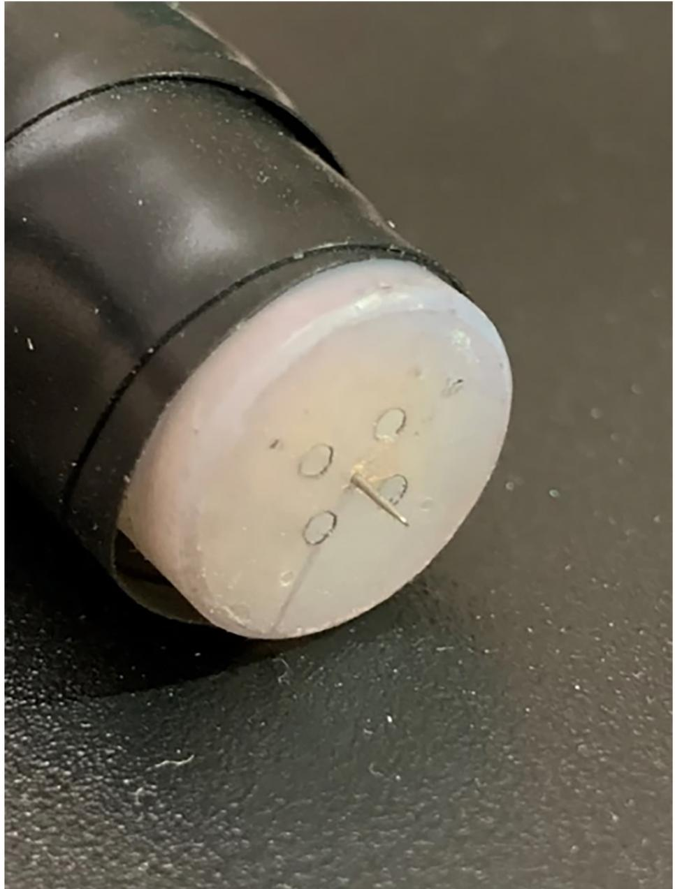
**Fig 3. Single needle electrode / corona generator [24].**
