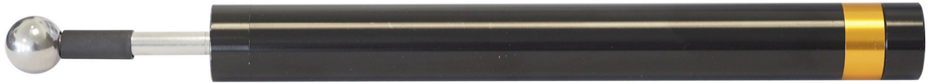
Fig 1. Pressure pain probe. Photo of a mechanical pressure probe, suitable for repeated pressure applications.
