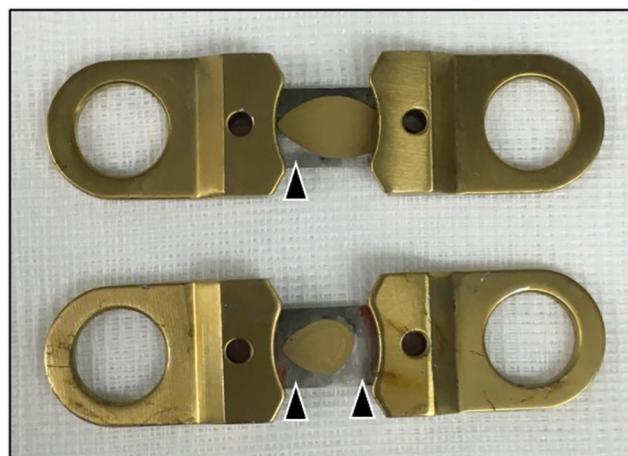
Fig 6. Explanted TiN coated stabilizers. Parts of the golden TiN coating are rubbed off at the region of contact surface with the bar, uncovering the underlying stainless steel (arrowheads). TiN = titanium-nitride.
