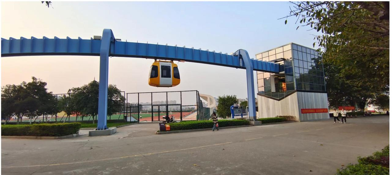
**Fig 1. Permanent magnet magnetic levitation rail transit system technology verification line.** Reprinted from [Jiangxi University of Science and Technology Permanent Magnet Magnetic Levitation Railway Transportation System Technology Validation Line] under a CC BY license, with permission from [Jiangxi University of Science and Technology], original copyright [2019].
