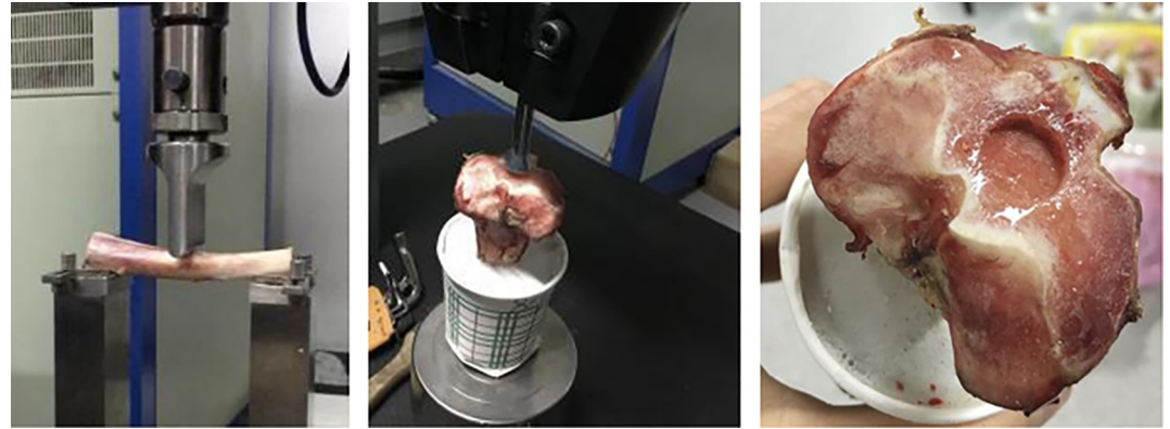
Fig 2. Mechanical testing. A. Three-point bending test. B. Indentation test. C. Proximal tibia after indentation test.
