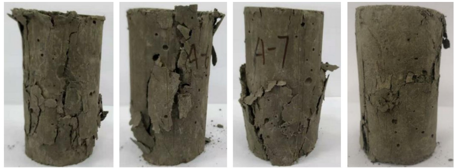
(a) 0.2% fiber content (b) 0.4% fiber content (c) 0.6% fiber content (d) 0.8% fiber content
