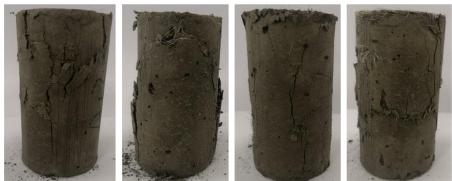
(a) 0.2% fiber content (b) 0.4% fiber content (c) 0.6% fiber content (d) 0.8% fiber content
